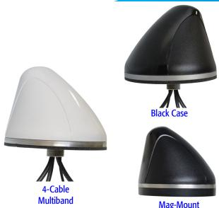
The SMW-413 Series Antennas features 4 elements in one antenna radome. The unique feature of this model is that the cellular element (Cable 1) is extremely widebanded and can cover: LTE at 700 MHz as well as the established 850/1900 GSM/CDMA bands, 1.7/2.1 GHz AWS and 2.5 GHz WiMAX all on a single board.
