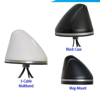
The SMW-305 Series Antennas features 3-elements in one antenna radome. The unique feature of this model is that the cellular element (Cable 1) is extremely widebanded and can cover: LTE at 700 MHz as well as the established 850/1900 GSM/CDMA bands, 1.7/2.1 AWS bands and WiMAX 2.5 all on a single board.
