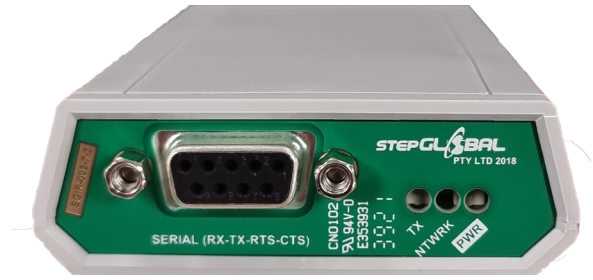
Back of unit with DB9 connector
