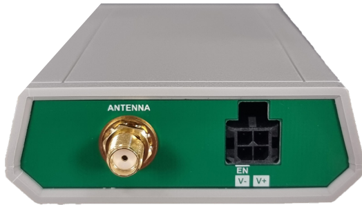
Front of unit with RF connection + Power
