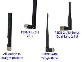
These half-wave rubber duck style device antennas require no ground plane for operation. This makes them ideal for use with portable devices or products with no substantial ground plane. They can even be used with products that are built with an all plastic chassis or case.
