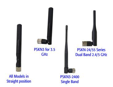
These half-wave rubber ducky style device antennas require no ground plane for operation. This makes them ideal for use with portable devices or products with no substantial ground plane. They can even be used with products that are built with an all plastic chassis or case.
