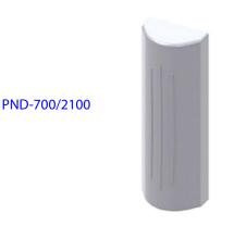
Mobile Mark's PND-700/2100 is a LTE Directional Panel Antenna with a dual-feed linearly polarized model. It offers 8 & 12 dBi gain, and covers 694-690 & 1710-2170 MHz. The corresponding beamwidths for this antenna ranges from 30° Elevation to 60° Azimuth.
