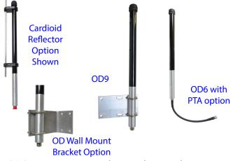
The OD Series antennas provide omni-directional coverage for WiFi 2.4 GHz applications. Four models are available from 3-12 dBi gain.
