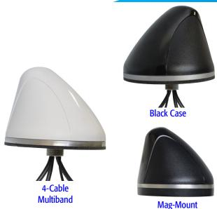
The SMW-410 Series Antennas features 4 elements in one antenna radome. The unique feature of this model is that it offers two identical high gain elements covering 2.4 GHz & 4.9-6.0 GHz. Of the remaining two elements in the SMW-410, one is used for GPS at 1575 MHz and the other covers 2.1-2.5 GHz & 4.4-6.0 GHz. All three elements offer an impressive 5 dBi gain.
